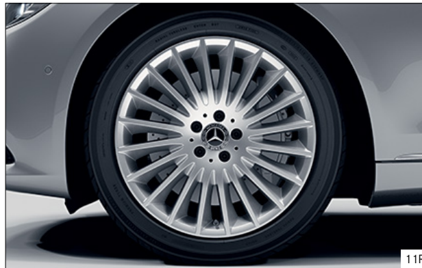
11R Multi-spoke light alloy wheels, vanadium silver, with 245/45 R 19 tyres at the front and 275/40 R 19 tyres at the rear (ex-factory accessory wheel; Standard for S 650)
