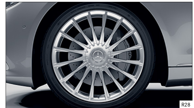
R28 Multi-spoke Maybach forged wheels, ceramic high-gloss polished finish, including fully integrated wheel bolt covers, with 245/40 R 20 tyres at the front and 275/35 R 20 tyres at the rear (Optional for S 650)
